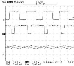
Figure 15 - Inductors current matching.
