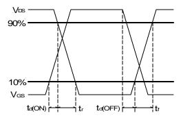
Figure 4 - Switching time waveforms.
