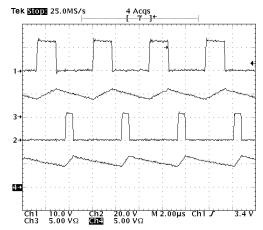
Figure 14 - Gate signals vs. inductor currents.
