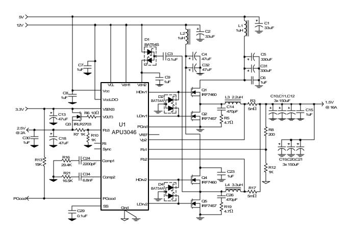
Figure 13 - Demo-board application of APU3046.
