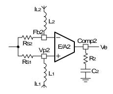
Figure 8 - The PI compensation network for slave channel.
