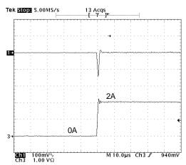
Figure 19 - Transient response for LDO @ lout = 0 to 2A.
