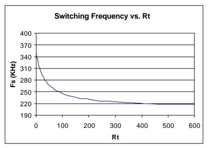
Figure 11 - Switching frequency per phase vs. Rt
